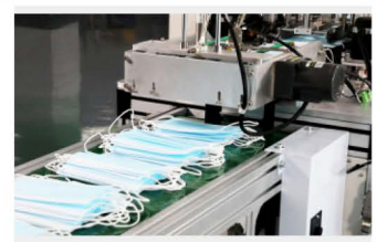
收料输送带机构 Collector conveyor mechanism
